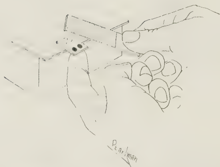
FIG. 281. Dry mounting of freeze-dried sections on Teflon support under dissecting microscope. Radioactive ● and non-radioactive control O sections are mounted simultaneously.
